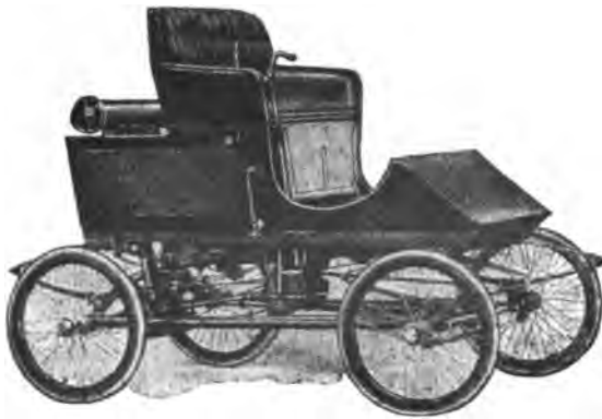
FIG. 153.—A "Toledo" Runabout. One of the well-known makes of American steam carriage using a water-tube boiler.
